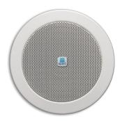
The CM4 is a stylish small built-in low impedance loudspeaker. Thanks to its halogen-spot size, it can be integrated into any interior style. It is ideal for speech and backgroundmusic in quiet areas, toilets, cloakrooms, ... The speaker has a full metal frame, a metal back can and a coated dual paper cone for the lowest distortion and increased resistance against moisture. The CM4 is easy to install thanks to its simple, quick mounting system (2 spring clamps).
